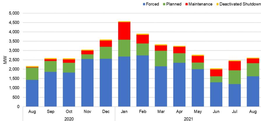
Average outage capacity in August continued to increase following the observance of higher forced and planned outage capacities while declining level of maintenance outage was observed. For ease of reference, Annex A shows the detailed information on plant outages in both categories.
