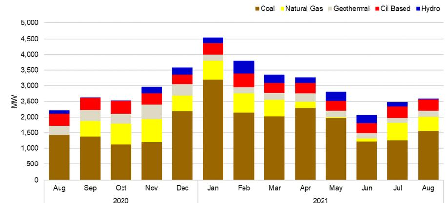
All plant types recorded increases in their averages except for natural gas and hydro plants. The most common reason for the forced outages of Coal power plants were due to emergency shutdown due to technical issues.
